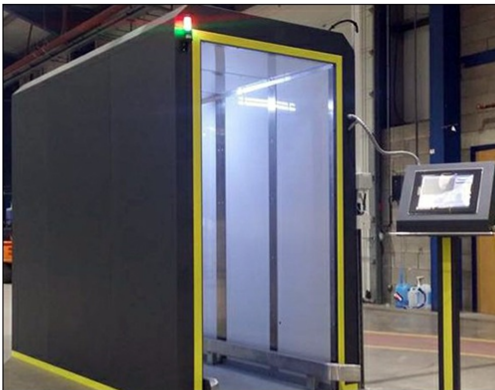
To document the arrival of soiled linens, Fishers installed an RFID portal made with an Impinj Speedway Revolution R420 reader and four circular-polarization antennas.
