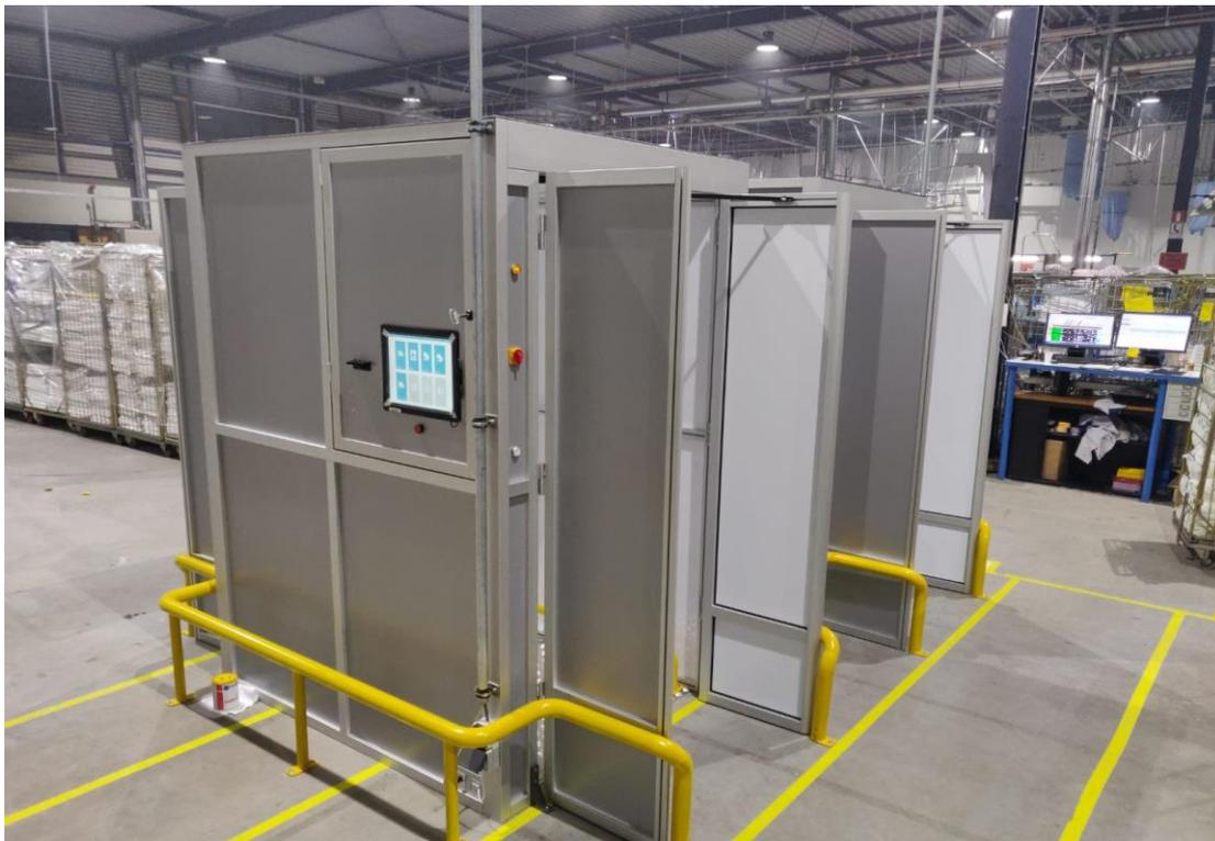
Figure 1 UBI Solutions closed door-Cabinet reading Units for Industrial Textile Industry
